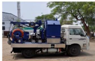
Jetting, grabbing, rodding machine (combination)
