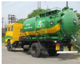
Gully emptier (Suction machine)
