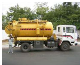
Hydro jetting machine
